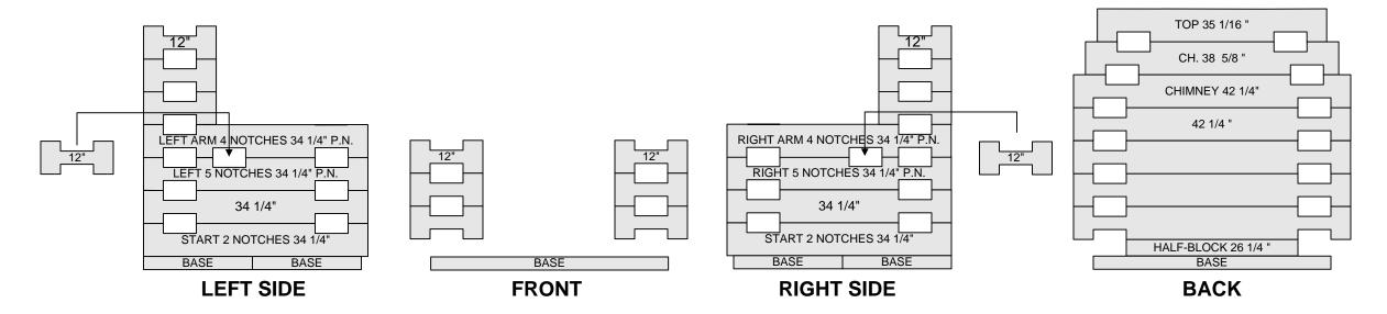
The flat side of each block must be put towards inside the fireplace. For greater security, we recommend the use of the Modular Pyramid Screen. Visit <a href="https://www.feuardent.com">www.feuardent.com</a> (Assembly section) for advices and assembly's pictures of your fireplace and the available accessories. For outdoor use only.
